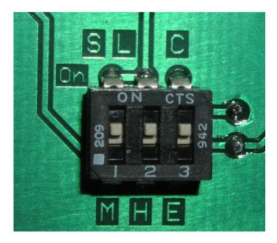
When the CW Machine is shipped, all three switches are in the ON position. The switch positions have single letter labels on the printed circuit board, describing their function. You can move the switches with a small screw driver or pen.
